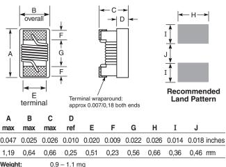
Tape and reel: 2000/7" reel 8 mm tape width
